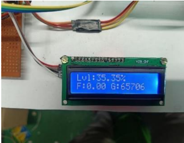
Fig. 4. Water level in LCD (Level)
